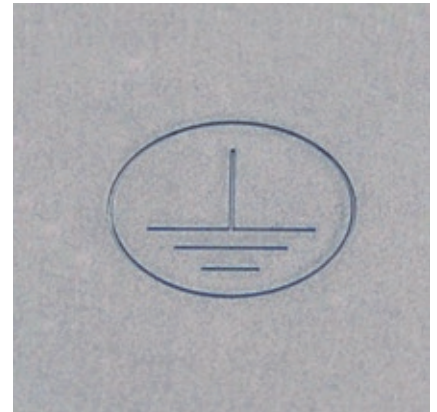
Ideal embossing – with adaptive stroke calibration
