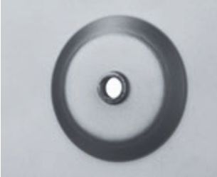
57. Cup with upward extrusion
