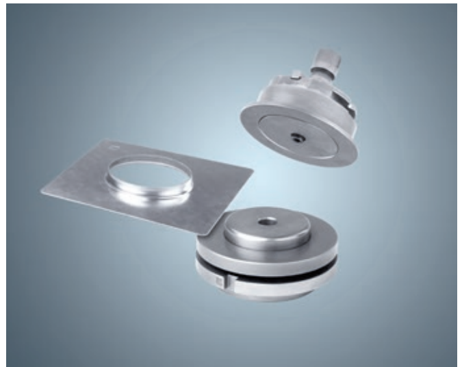
Extrusion tool size 5 for the active die
